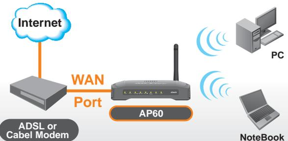
In this mode, the AP behaves like a normal wireless router. You can connect the Internet line from ADSL Modem or Cable Modem to the WAN Port.
