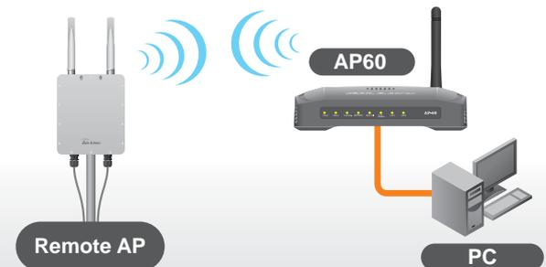
The WDS Station mode is similar to Bridge mode with the exception that the link has added "SSID" as basis for the bridge link.
